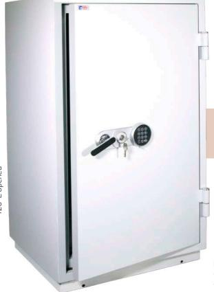
Series of safes certified according to European standard LFS 60P EN15659 for fire resistance. Designed to protect documents, since the temperature increase inside the safe at 60 minutes is less than 170°, which guarantees the integrity of the paper, which decomposes from 177°C. Also ideal for storing valuable belongings that must be protected from theft.
